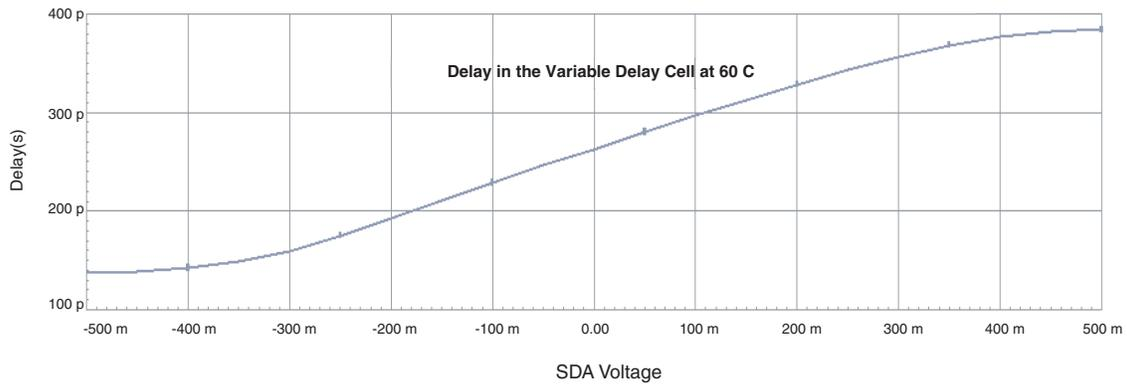
The variation of the delay in function of the temperature is negligible. If this function is not used, SDAEN can be left floating as well as the SDA pin.
