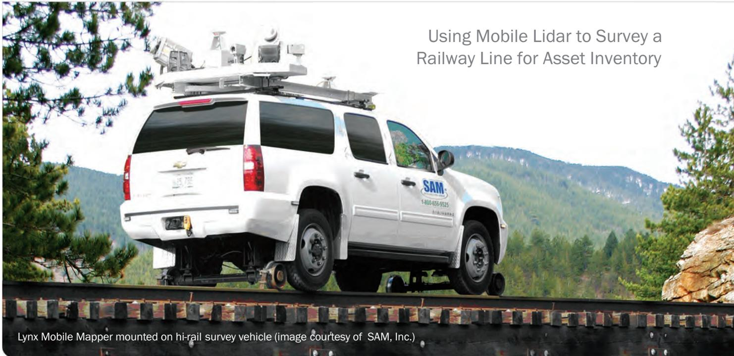
Using Mobile Lidar to Survey a Railway Line for Asset Inventory
