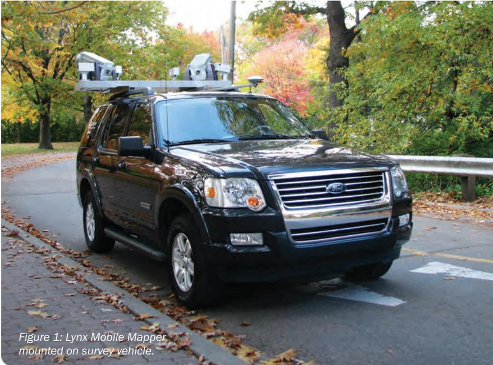
Figure 1: Lynx Mobile Mapper mounted on survey vehicle.
