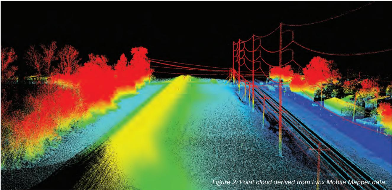
Figure 2: Point cloud derived from Lynx Mobile Mapper data.
