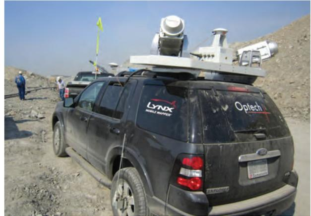
Lynx Mobile Mapper mounted on survey vehicle at an open pit mine
