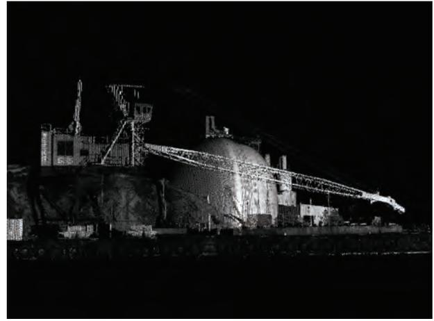
Lidar image of unloading facility
