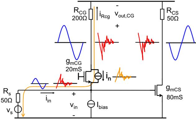
Fig. 1 The Balun-LNA, a combination of a Common Gate (CG) and admittance scaled Common Source (CS) stage to realize simultaneous output balancing, noise and distortion canceling
