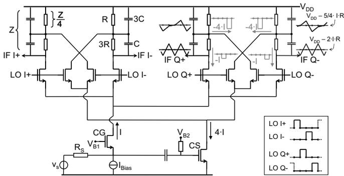
Fig. 2 A Balun-LNA with I/Q down-converter exploiting the CG-CS stage of Fig.1.
