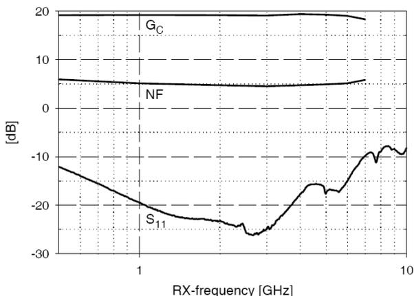
Fig. 3 Gain, Noise figure and  $S_{11}$  of a 65nm CMOS IC shown in Fig. 2. Note that the high and flat gain is achieved at only 1.2V supply.
