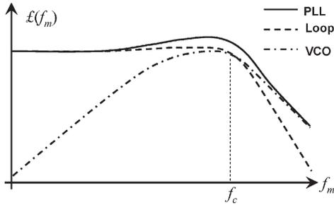
Fig. 2. Overall PLL output phase noise with  $1/f$  noise neglected.
