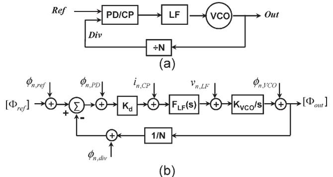
Fig. 1. Classical PLL (a) architecture and (b) phase domain model.
