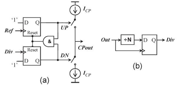
Fig. 3. Schematic of (a) a three-state PD/CP and (b) a divider with synchronization.
