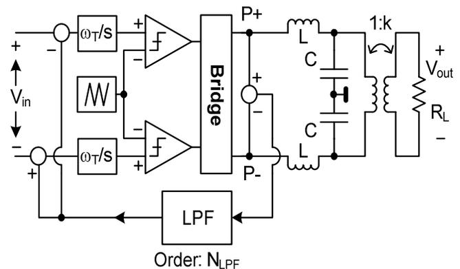
Figure 1: Block diagram of 3-level PWM line driver.
