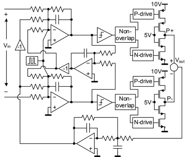
Figure 4: Single-ended representation of line driver.
