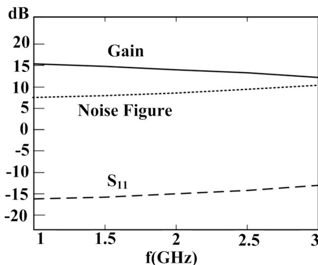
Figure 4.4.4: Gain, S<sub>11</sub> and Noise Figure per channel.
