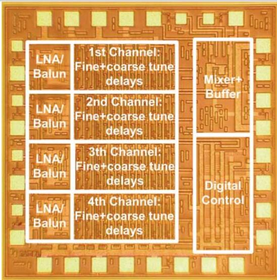
Figure 4.4.7: Photograph of the chip, measuring 1.0x1.0mm<sup>2</sup>.
