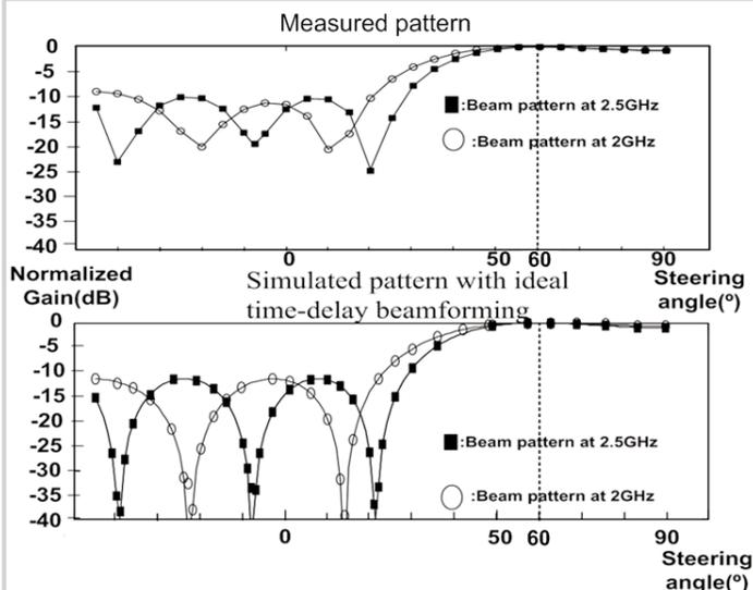
Figure 4.4.5: Beam patterns for 60° beam direction.
