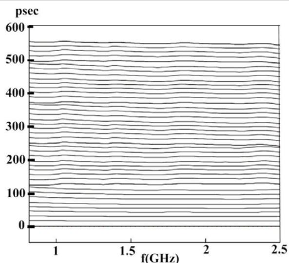
Figure 4.4.3: Measured delay for all delay settings.
