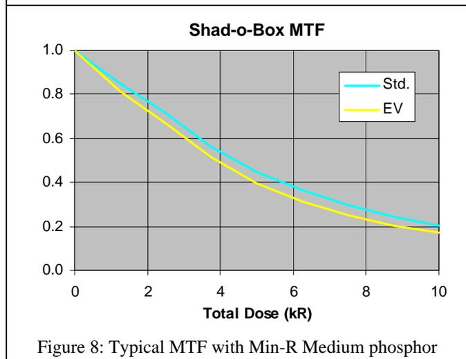
Figure 8: Typical MTF with Min-R Medium phosphor
