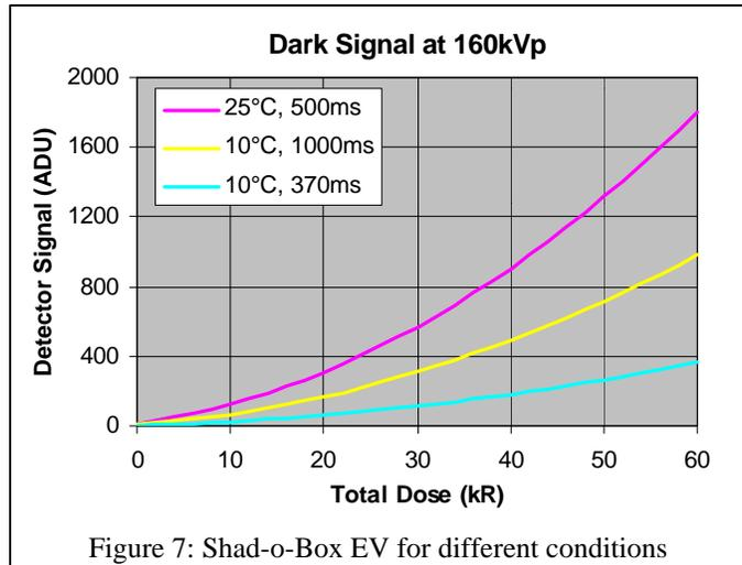
Figure 7: Shad-o-Box EV for different conditions
